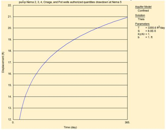
If pumping 200 gpm is simulated for 69 days for 20 million gallons as proposed in the new application and then continue on with 49 gpm for the remainder of the year for 296 days for 21 million gallons, drawdown spikes a foot or two at 69 days but by the end of 365 days total drawdown is only about a half-foot greater or 21.4 feet.
