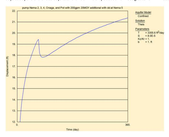
In the previous analysis the Woolsoncroft well caused a simulated drawdown of 31 feet at Nema well 5, the other Wooloscroft well simulated caused 18 feet drawdown but that is proposed to be dismissed. So with the Nema well 5 pumping, and all other municipal wells pumping, simulated drawdown would still leave about 112 ft of available drawdown at Nema well 5 even with the proposed additional pumping from Pot well 4.
