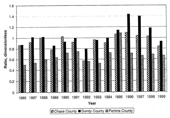
Figure 3b. Ratios of Pumpage to Crop Irrigation Requirement for Center Pivot Irrigated Corn.
