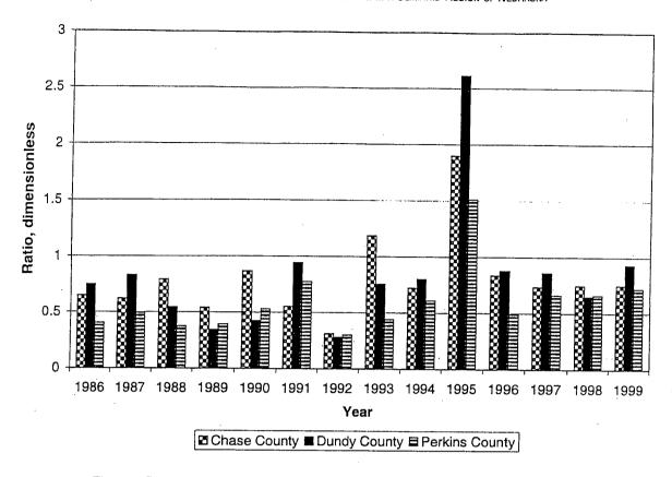
Figure 3c. Ratios of Pumpage to Crop Irrigation Requirement for Center Pivot Irrigated Wheat.
