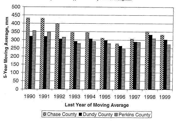
Figure 5a. Five-Year Moving Average of Pumpage for Gravity Irrigated Corn.
