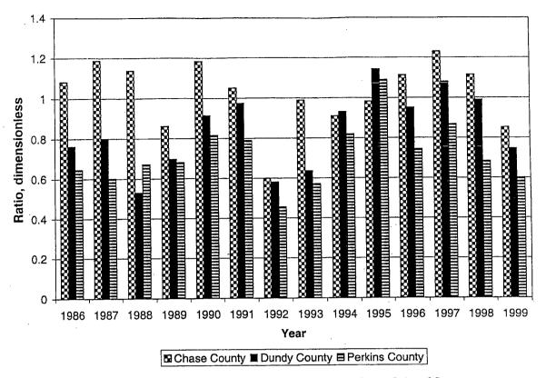
Figure 3a. Ratios of Pumpage to Crop Irrigation Requirement for Gravity Irrigated Corn.
