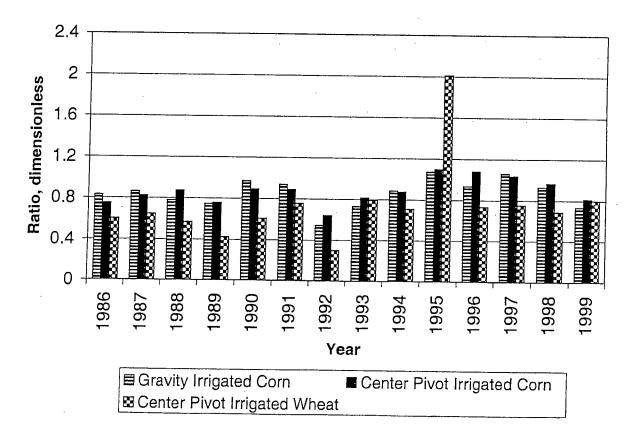
Figure 6. Means of Pumpage to Crop Irrigation Requirement Ratios for Three Counties.
