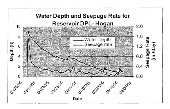
Seepage = Rain fall + Runoff - Evaporation - Overflow  $\pm \Delta S$
