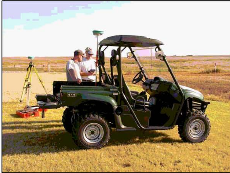
Figure 3. Picture of the all terrain vehicle and survey-grade GPS system used to survey terrace conditions.
