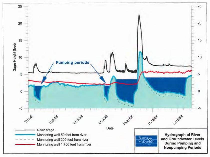
Note: Pumping was started on September 23, 1998 and ended on December 17, 1998. Well pumped a total of 117 million gallons over 86 consecutive days. Groundwater Levels were 3 feet higher than before pumping started. All water levels were recorded and reported by USGS personnel.
