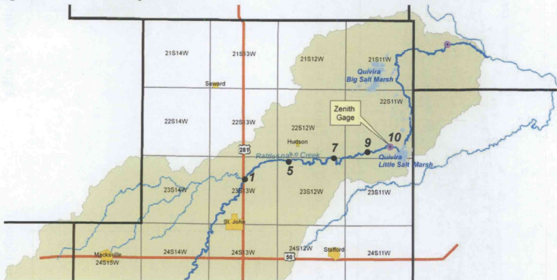
Figure 5: Chloride sample and flow measurement locations on Rattlesnake Creek
